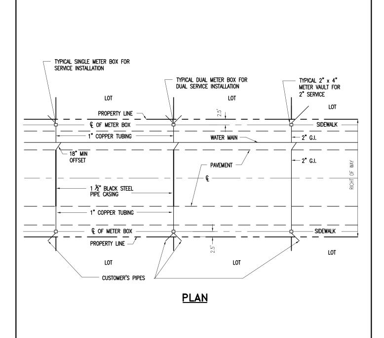
$\underline{\mathsf{NOTE}}\textsc{:}$  Meters will not be installed if the meter box is in a driving surface.
