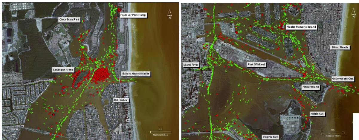
Figure 28a. Composite view of vessel traffic data from all 20 aerial survey flights are combined. Green arrows indicate vessels underway. Red dots indicate stationary vessels.
