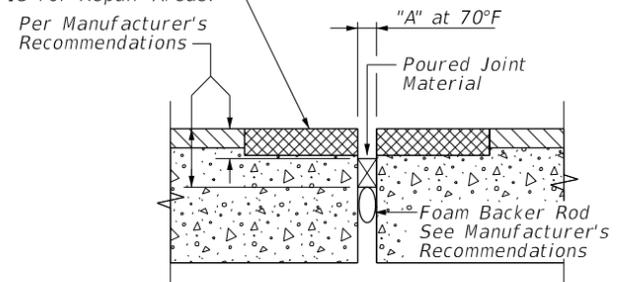
**TYPICAL SECTION THRU JOINT**
