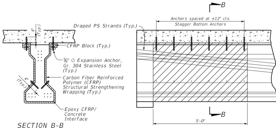
**CARBON FIBER REINFORCED POLYMER (CFRP) STRUCTURAL STRENGTHENING WRAPPING DETAILS**
