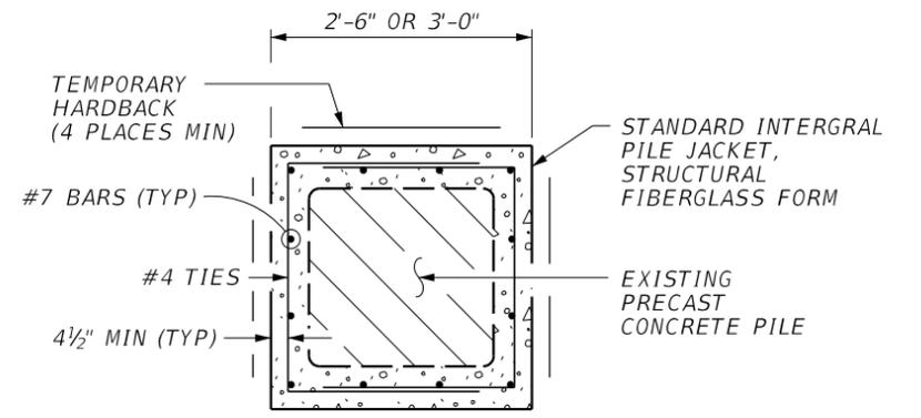
**SECTION A-A THRU PILE JACKET**
