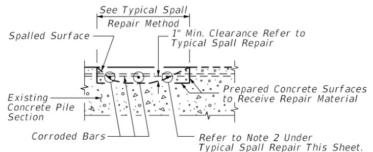
**EXPOSING AND UNDERCUTTING REINFORCING STEEL**
